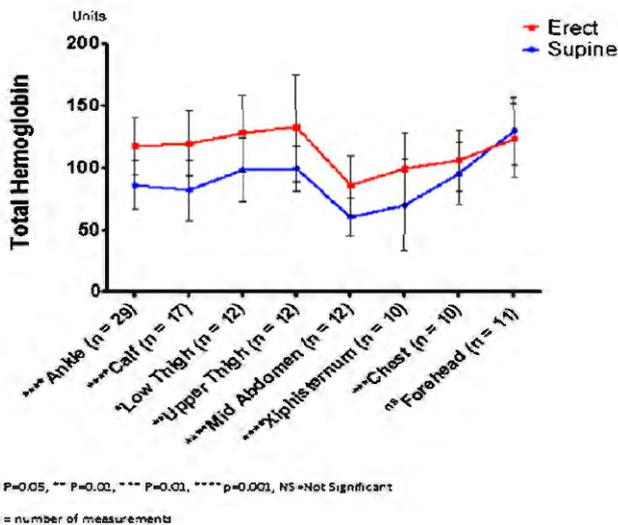
Figure 3. Regional variations in orthostatic microvascular congestion derived from OxyVu-2™ data: Note significant increase in hemoglobin content in the lower part of the body up to the xiphisternum on assuming the erect position.
