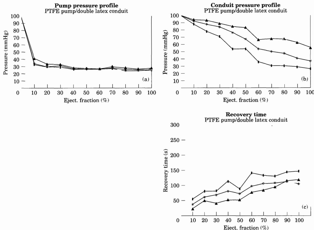
Fig. 5. Pressure profile in the pump (5a), the conduit (5b) and recovery time (5c) in response to volume changes in the pump for PTFE pump/2-ply latex conduit combination. (■) 1% valve O; (\*) 5% valve O; (▲) 10% valve O.
