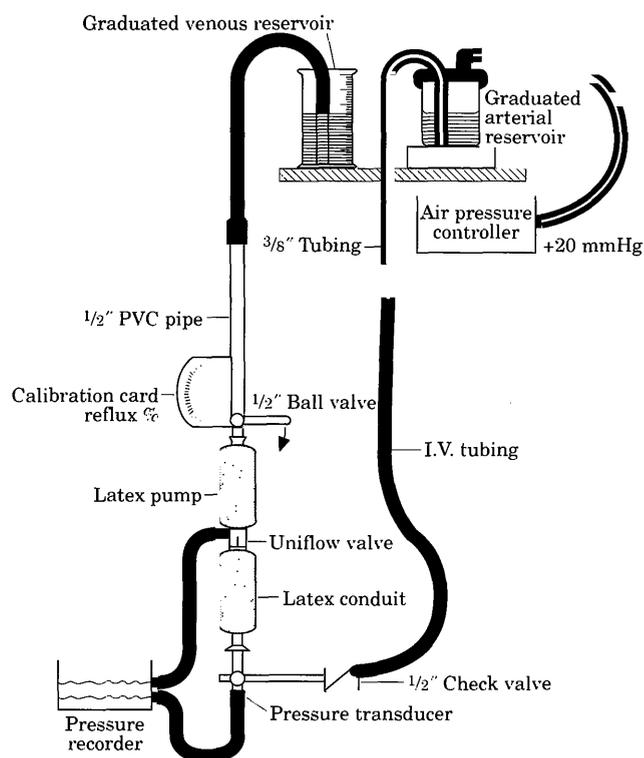
Fig. 1. Two-valve, two-tube model utilised in the study. See text for description.
