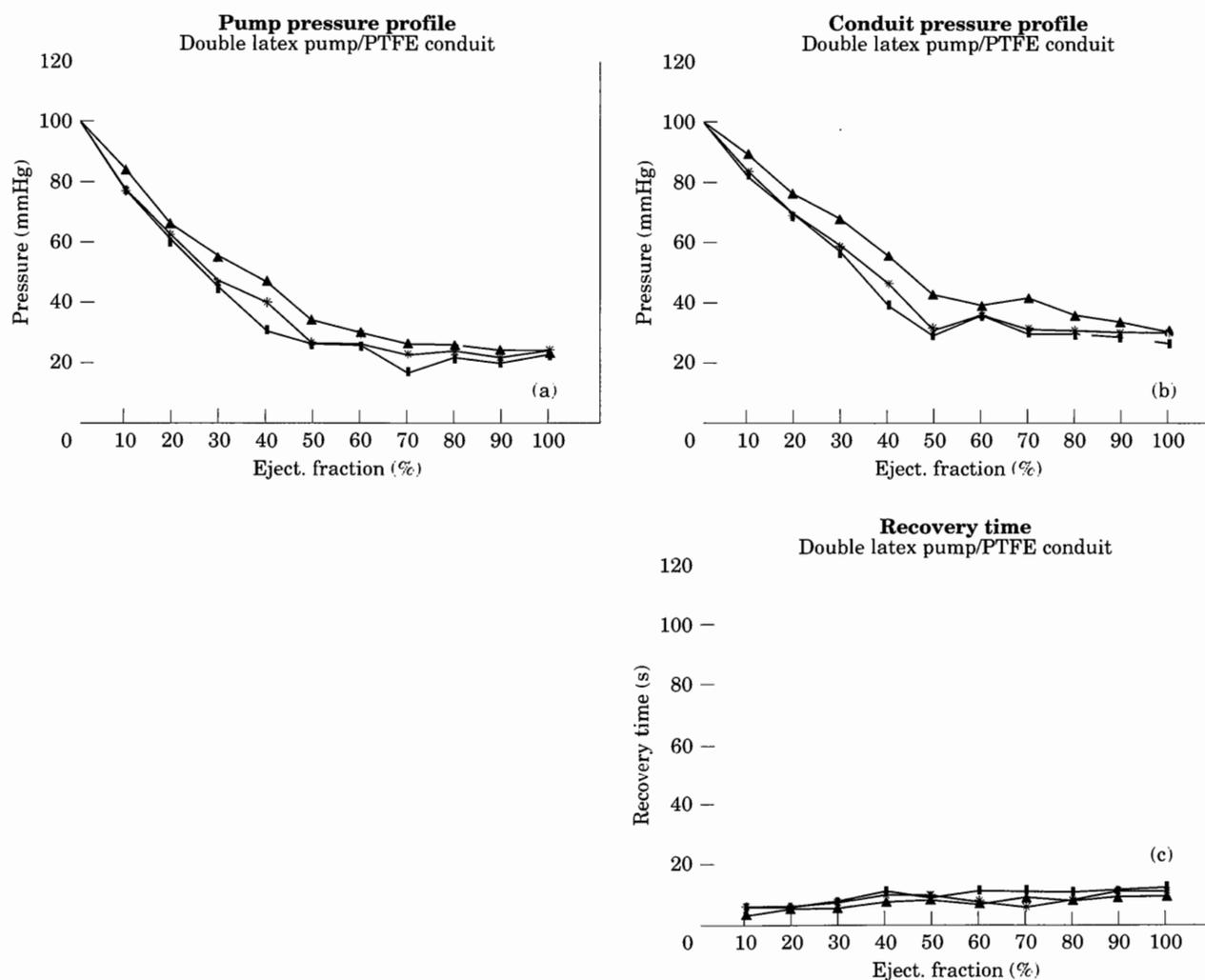
Fig. 6. Pressure profile in the pump (6a), the conduit (6b) and recovery time (6c) in response to volume changes in the pump for 2-ply latex/PTFE combination. (■) 1% valve O; (\*) 5% valve O; (△) 10% valve O.
