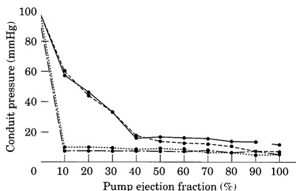
Fig. 2. Comparison of volume pressure curves for 1% valve leak in the pump when materials of different compliance were utilised in the pump. (—) Double latex; (- - -) polyethylene; (· · ·) quad latex; (- · - ·) PTFE.
