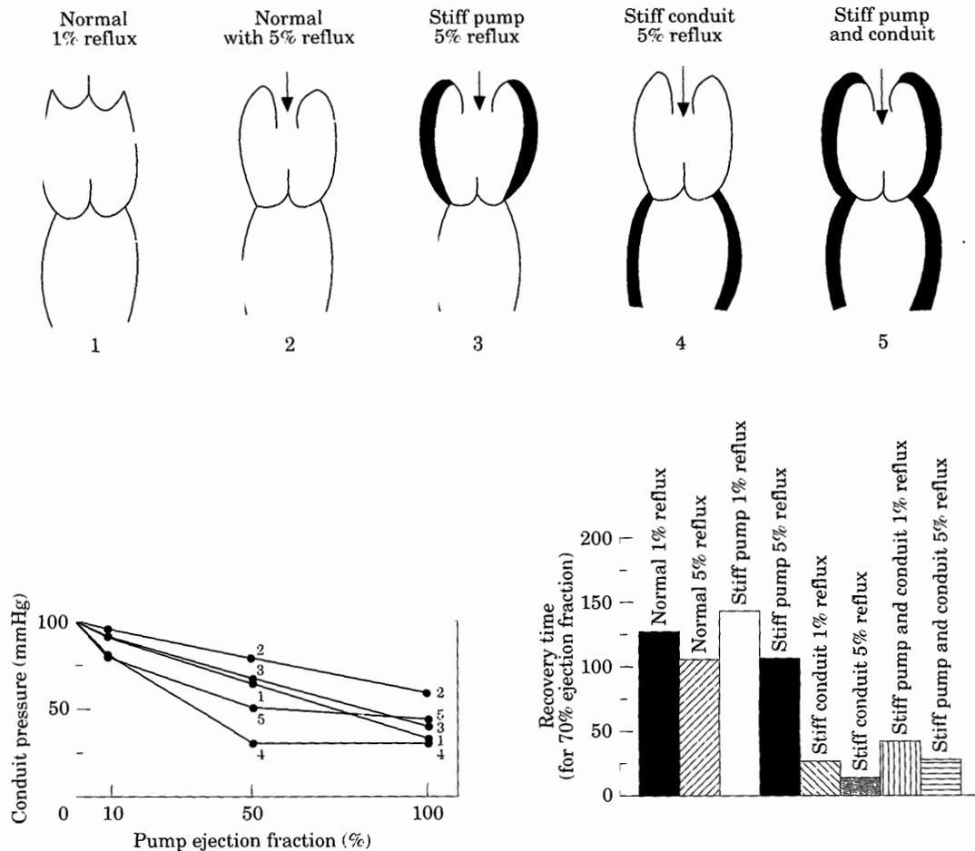
Fig. 9. Comparative conduit pressure profile and recovery times (bottom) (for 70% ejection fraction) for various pump/conduit combinations (top). Stiff pump or conduit = PTFE. A stiff conduit exhibits a paradoxical decrease in conduit pressure with a more profound depression of recovery times compared to a stiff pump. Reflux has a relatively minor effect on recovery time compared to conduit compliance.
