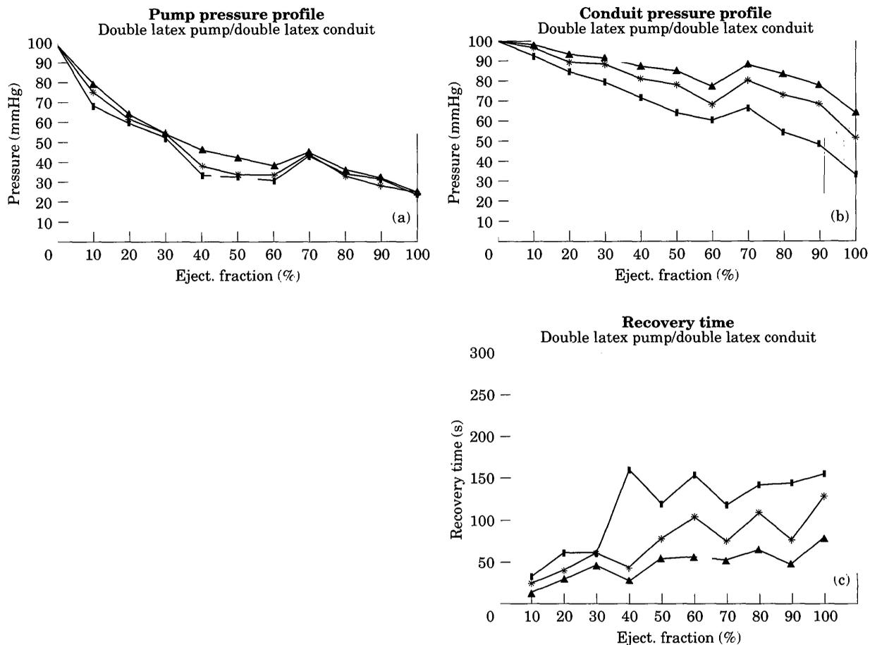
Fig. 3. Pressure profile in the pump (3a), the conduit (3b) and recovery time (3c) for the basic 2-ply latex/2-ply latex model. (■) 1% valve O; (\*) 5% valve O; (▲) 10% valve O.
