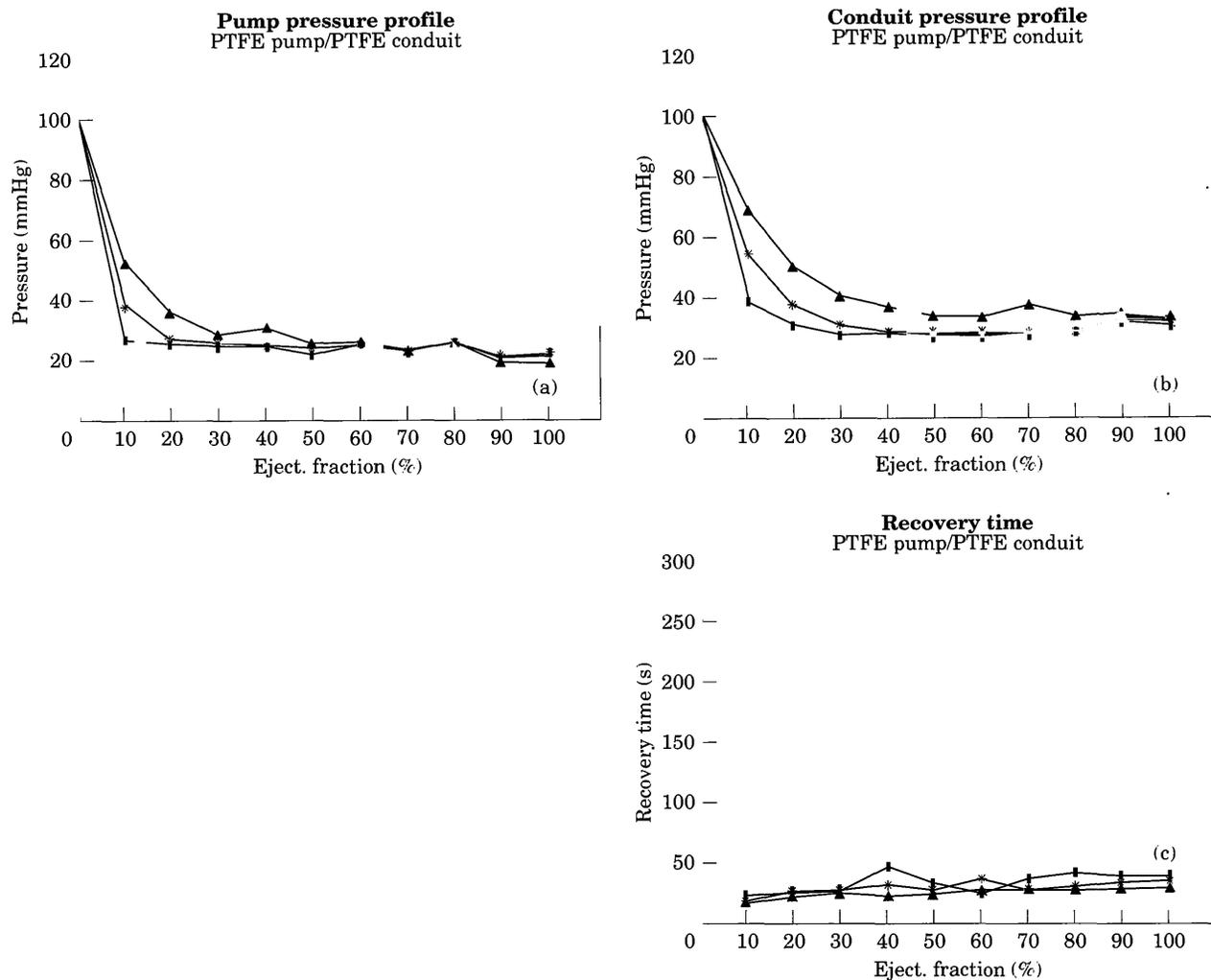
Fig. 7. Pressure profile in the pump (7a), the conduit (7b) and recovery time (7c) in response to volume changes in the pump for PTFE pump/PTFE conduit combination. (■) 1% valve O; (\*) 5% valve O; (▲) 10% valve O.
