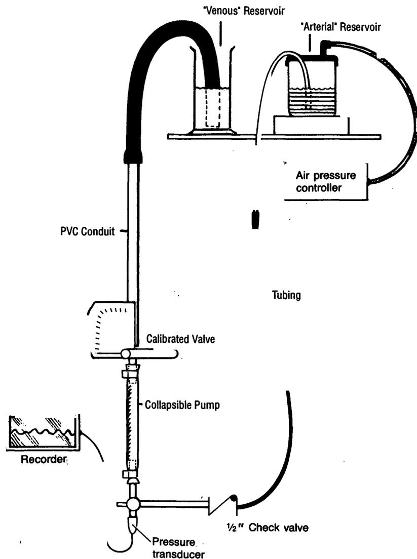
Figure 1 ♦ A schematic diagram of the mechanical model utilized in the experiment.
