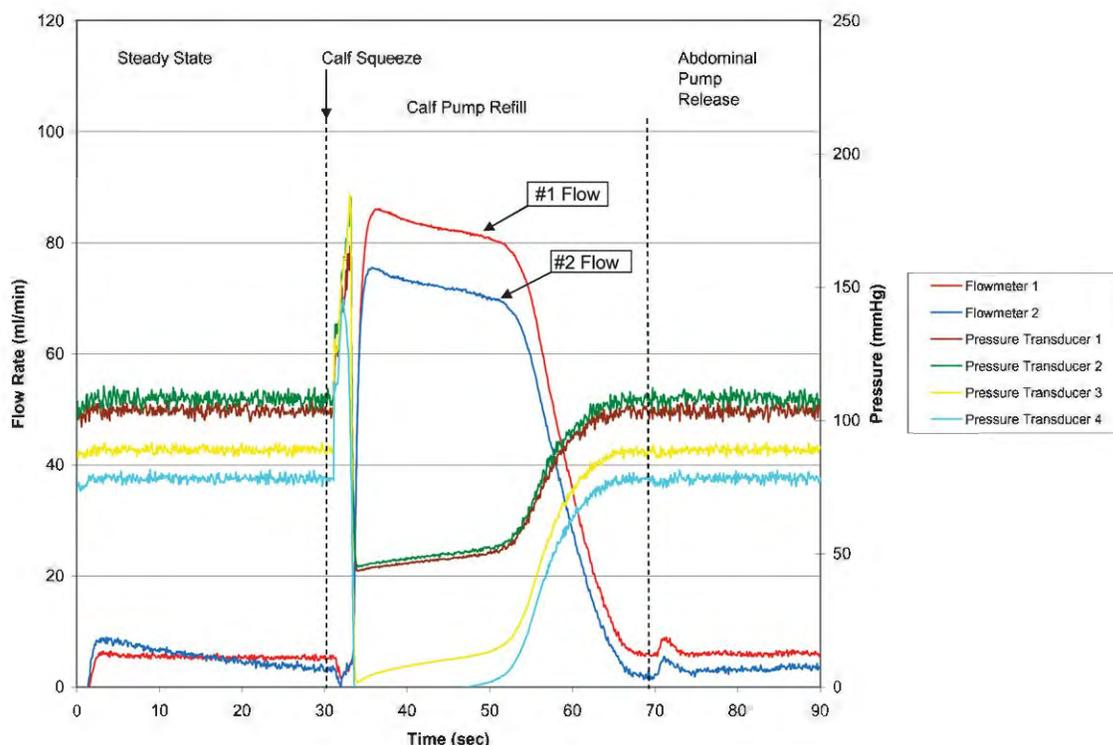
Fig. 2. Basal flow. Flow curves for identical base pressure head setting of 15 mmHg (zero pressure differential) at the reservoirs with abdominal compression of +5 mmHg. Note huge augmentation of flow rate (velocity) during calf pump refill increasing several folds from the steady state flow. Calf pump pressure (yellow line, right scale) falls to near zero.
