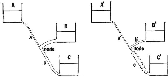
**Fig. 5.** Flow dynamics between three interconnected reservoirs. *Left:* Classic three-reservoir problem with rigid conduits. EGL relationships at the node determine whether reservoir B will flow outward or receive inflow from reservoir A. *Right:* Modification of flow with collapsible conduits: The presence of a collapsible tube in conduit *c'* (calf pump in the model) allows for dynamic change in EGL relationships at the node influencing flow behaviour of reservoir B'. See text.
