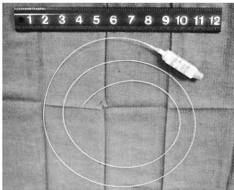
**Fig 1.** The Millar probe.
