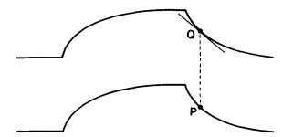
**Fig. 1.** Typical plethysmographic volume (*top*) and dorsal foot vein pressure (*bottom*) curves. Flow Q can be calculated from tangent on volume curve at any point and corresponding pressure P measured. Resistance is determined as P/Q.
